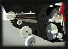
The dosing rate is easy to set by changing gears. Spare gears are standard included. Dosing starts from 1,4 gr/m<sup>2</sup> (0.3 lbs/1000)
