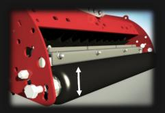
The hole depth can be changed by adjusting the rear roller up and down
