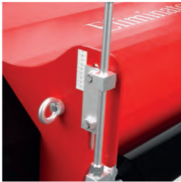
Simple and accurate adjustment of working depth.
