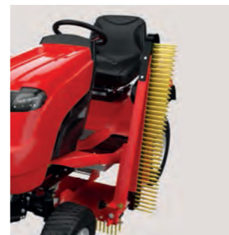
Folding wings to allow access.
