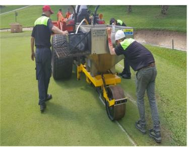
With the patented modified sandbander, installation is quick and seamless with no excessive excavation, complicated pipe maintenance, and expensive french drain work. Our Installation technique doesn't require shutting down for long periods of time and ensures playability within 24 hours
