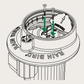
2. Align the adjustment ports on sod cup with the adjustment screws on rotor. Place sod cup on top of rotor and secure with screws.
