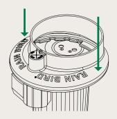
1. Align wide tab on flange cover with wide space on case and press flange cover onto case.
