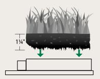
3. Using a standard golf-hole cutter, cut a sod plug. Place small slice in the center of the plug to accept the pull up tab. Install sod into cup and press firmly into place.
