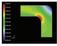
Figure 3: Swing Joint Pressure Loss
