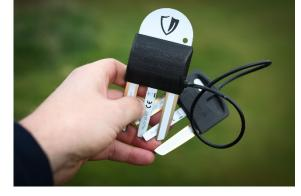
The master Hydra sensor takes care of all radio communication, just like before. It can be buried in shallow ground to give an excellent range, whilst querying subsoil data from the second sensor, deep down in the same hole.
