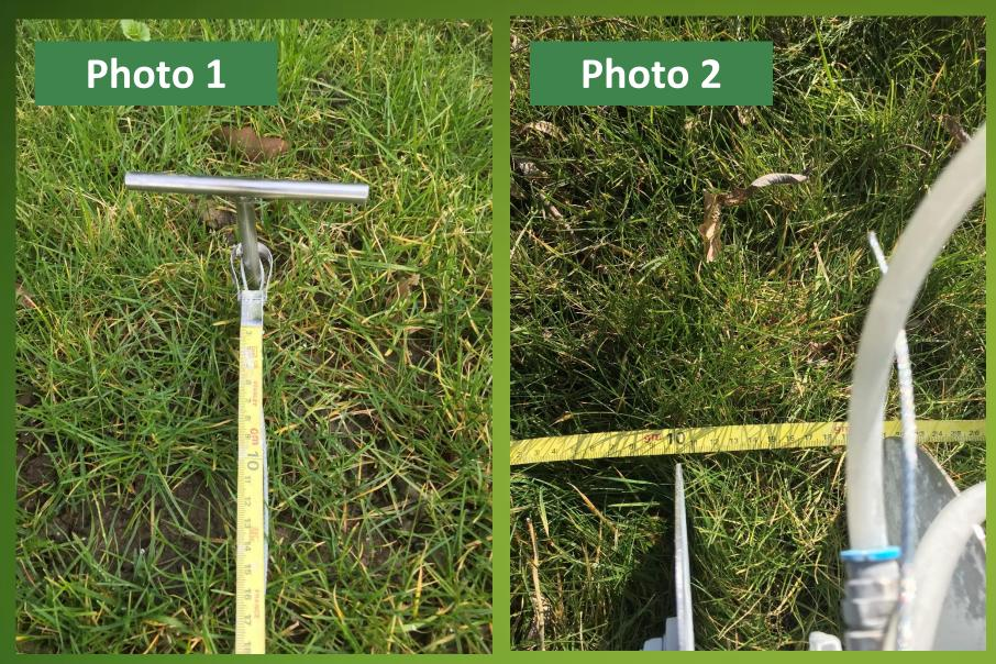
Use a tapeline to put the nozzle at 9 m 15 distance from the peg at the center circle (Photo 1 and 2).
