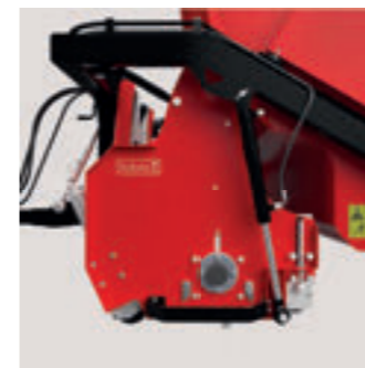
Floating head to manage undulations.
