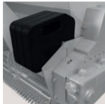
Optional weights can be added for harder ground conditions.
