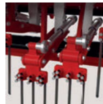
Unique drawrod design to give speed and precision.
