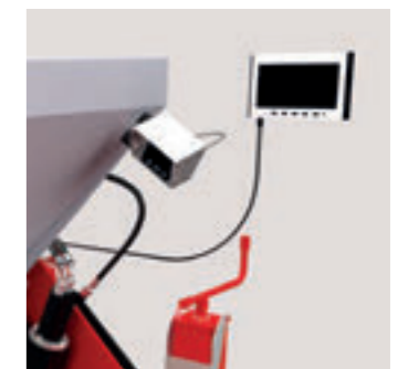
Camera to monitor the filling area.
