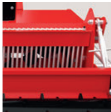
Screening fingers can be altered for different material types and finishes.
